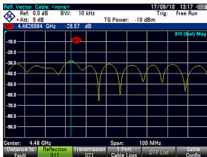
Figure 2-2: Results of a reflection measurement
