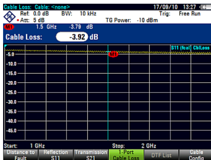
Figure 2-4: Results of a cable loss measurement
